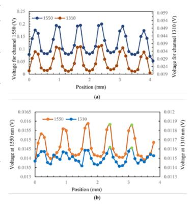
Figure 8: Measured voltage signal at both channels versus position conducted with pyrometer: (a) MMF; (b) SMF, green dots show data with negligible effect of noise in both channels.
