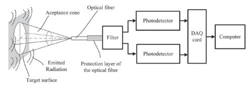
Figure 2: Experimental two-color optical fiber pyrometer set-up [20].
