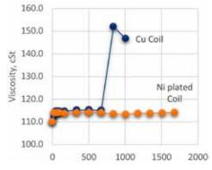
Figure 4: Kinematic viscosity testing per ASTM D445 for the copper coil and nickel-plated coil.
