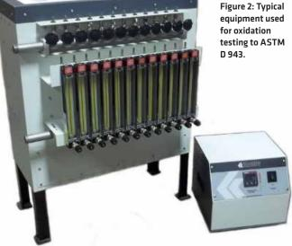
ture, is heated in the presence of a copper coil. An example of this equipment is shown in Figure 2.
