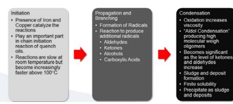
Figure 1: Schematic representation of the progression of oxidation.
