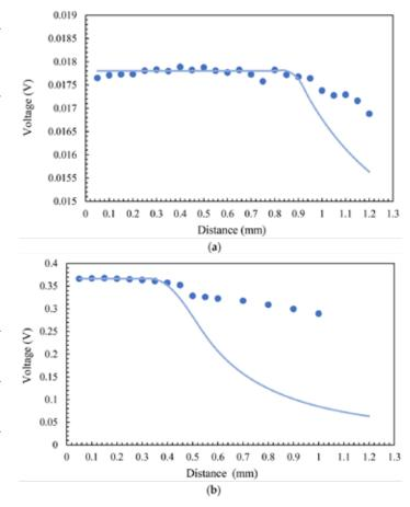
Figure 7: Experimental (dots) and theoretical (lines) voltage in channel 1,550 nm vs. distance from an object with a diameter of 0.25 mm for (a) SMF, and (b) MMF.
