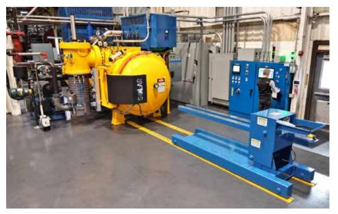
A recently commissioned Solar Atmospheres vacuum furnace has a working hot zone of 24" x 24" x 72" deep and uses several unique hot zone design features to increase the quench rate. (Courtesy: Solar Atmospheres)
