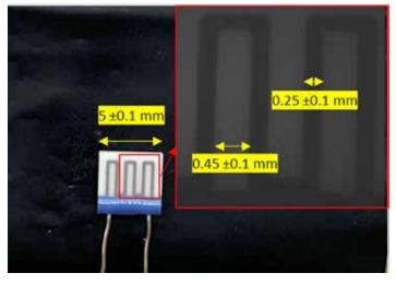
Figure 3: The commercial microheater and its pattern, which was acquired using an optical microscope at 100× zoom.
