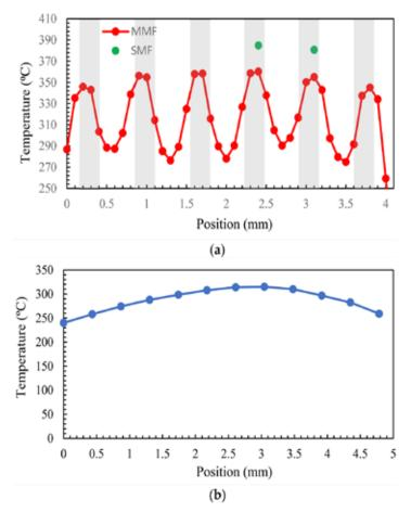
Figure 9: Temperature measurements with the micrometer in different positions with: (a) high spatial resolution optical fiber pyrometer; (b) thermal camera. Shadow lines show the microheater pattern.
