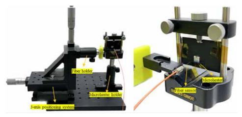
Figure 6: The experimental set-up with fiber and microheater holders and the positioning system.
