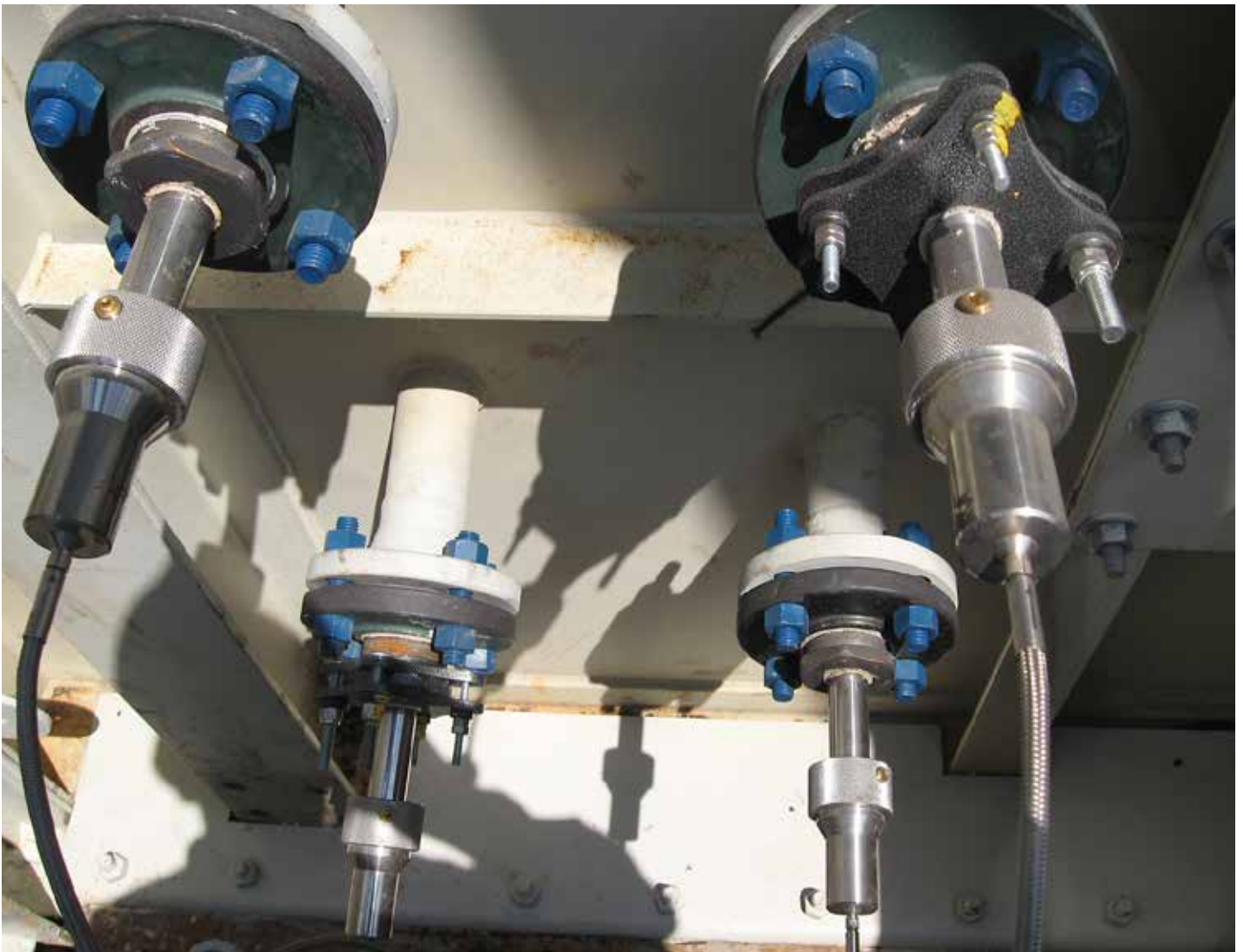
An EXACTUS® pyrometer used for furnace temperature measurement. (Courtesy: BASF ECMS)
