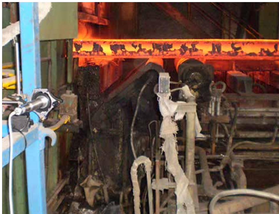
Heat monitoring with EXACTUS® in a rolling mill reheat process. (Courtesy: BASF ECMS)
