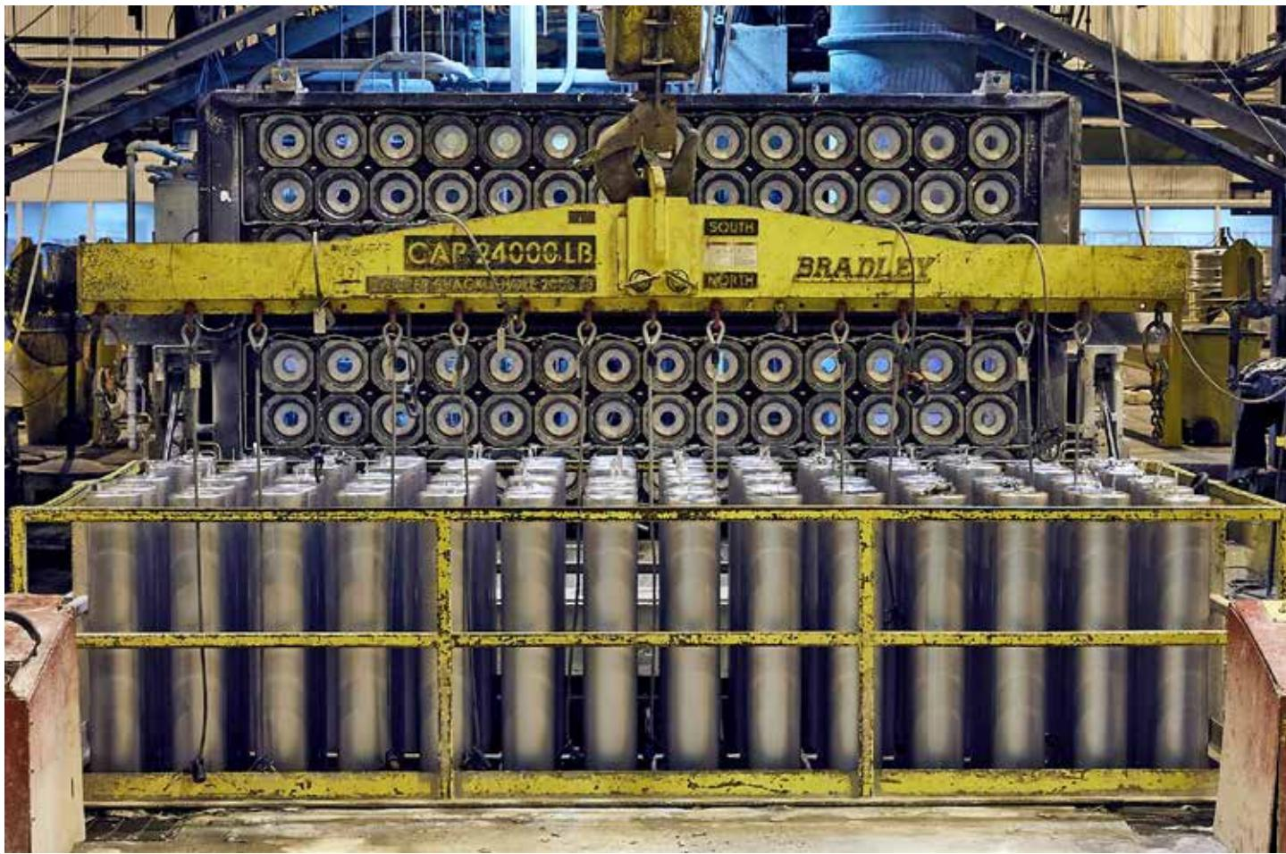
Century Aluminum's Mt. Holly plant produces about 70 alloy combinations, with custom ordering available, including billet, horizontal direct chill (HDC) ingot, T-ingot, and slab aluminum. (Courtesy: Century Aluminum)
