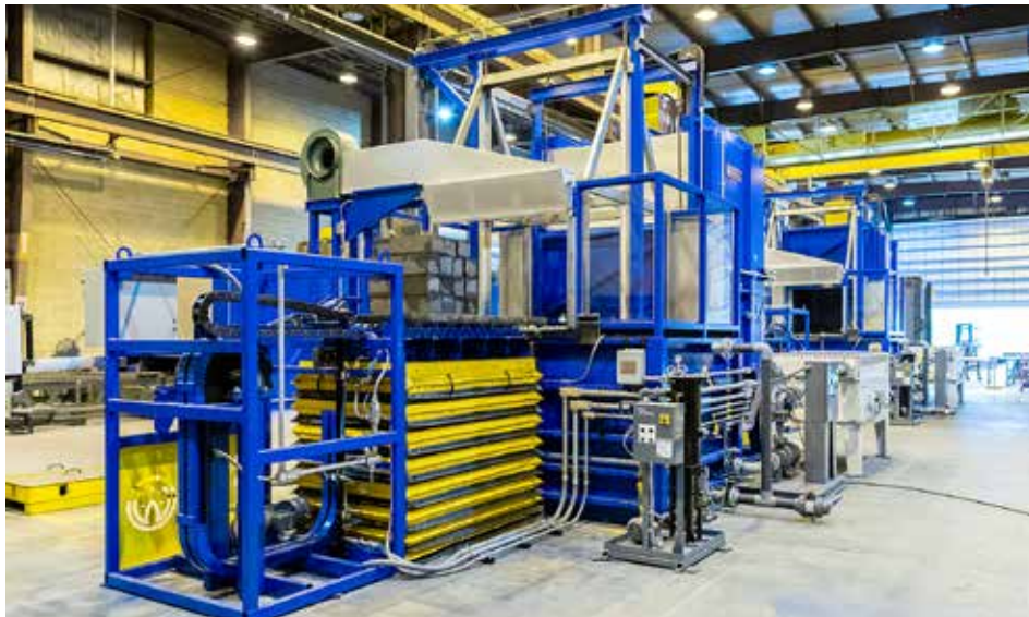
Each recently shipped Wisconsin Oven horizontal quench furnace has a maximum temperature of 1,250°F, and capacity to heat and support a 4,500-pound gross load. (Courtesy: Wisconsin Oven)
