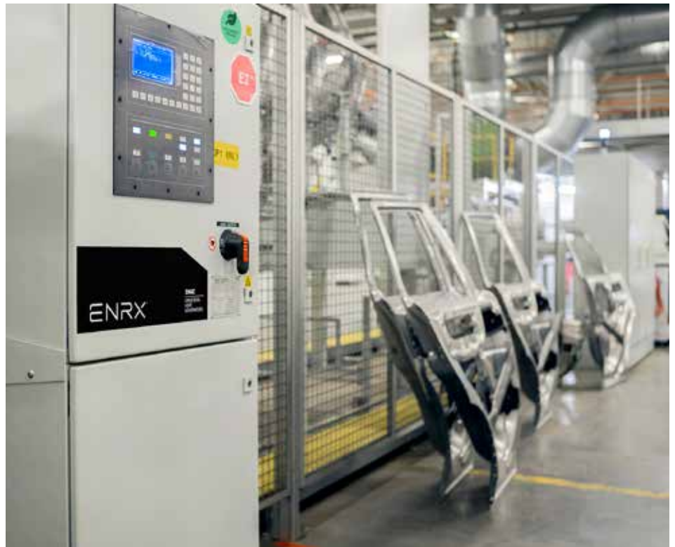
Induction heating can be used for metal heat treatment of almost any body panel, chassis, driveline, electrical, or engine part of a vehicle. (Courtesy: ENRX)
