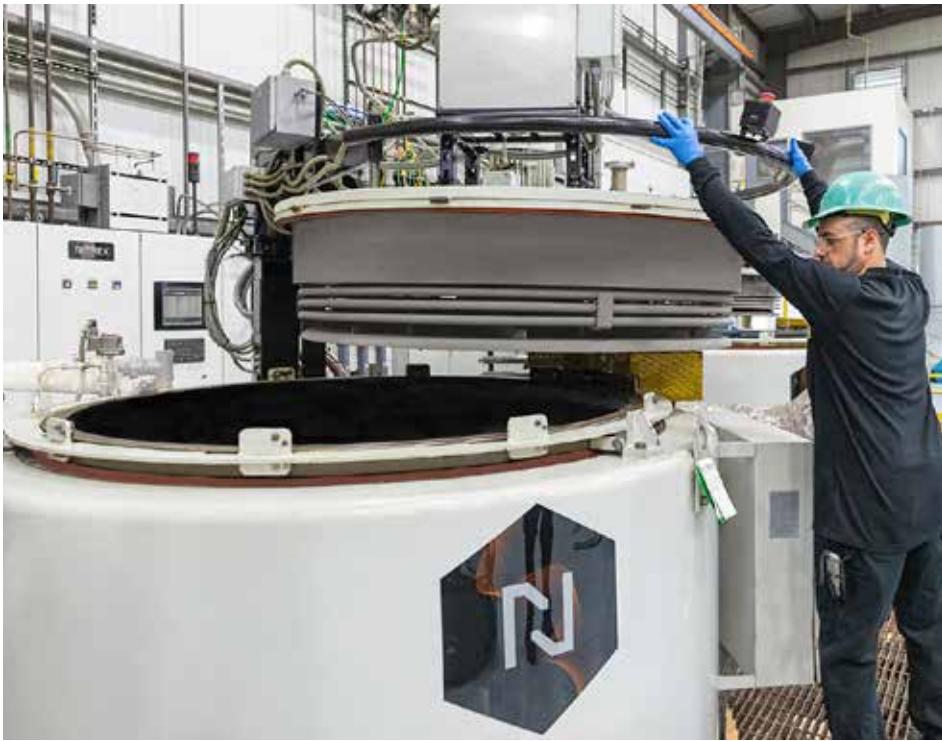
Castool Tooling System's new pit-type nitrocarburizing furnace, a Nitrex model NX-1625 is capable of processing large workloads of up to 6,000 kg. (Courtesy: Nitrex)
