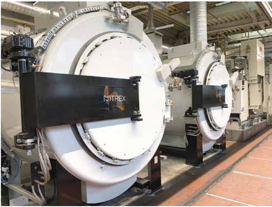
A European hydraulics manufacturer strengthened its in-house heat-treatment capabilities with a second set of nitriding/nitrocarburizing systems from Nitrex. (Courtesy: Nitrex)
