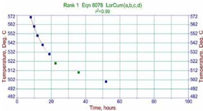
Figure 3: Effect of nitriding temperature and time for producing 0.015" total case depth in 4340 steel.
