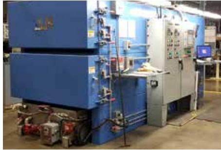
Delta H ® Model DCAHT ® -3016120-1200/1200-BAC provides tamperproof batch records, simple performance of the temperature uniformity survey (TUS) and the system accuracy test (SAT), and requires minimal maintenance. (Courtesy: Delta H)
