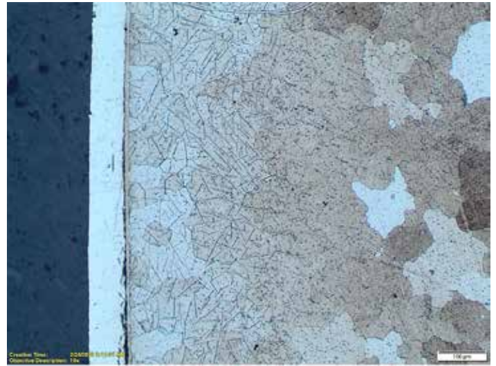
Figure 9: Structure of nitrided/diffusion layer in 1215 steel. Etched with 3% Nital.
