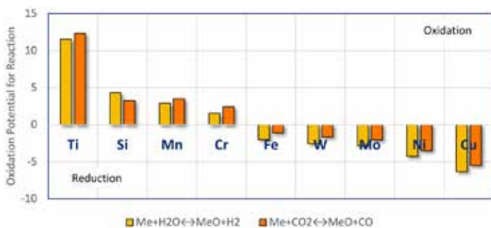
Figure 2: Oxidation potential of alloying elements in steel heated in an endothermic atmosphere [7].
