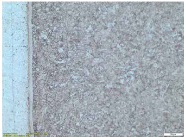
Figure 1: Nitrided layer produced in 4340 steel after the ion/plasma nitriding process at two different magnifications. Etched with 3% Nital. White layer on the left is a nickel foil used for better edged retention.
