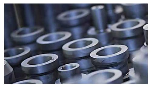
Carburizing is a thermochemical process in which carbon is diffused into the surface of low carbon steels to increase the carbon content to sufficient levels so the surface will respond to quenching and produce a hard, wear-resistant layer.
