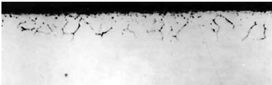
Figure 1: Unetched optical micrograph showing surface oxidation in a gas carburized SAE 4320 [3].
