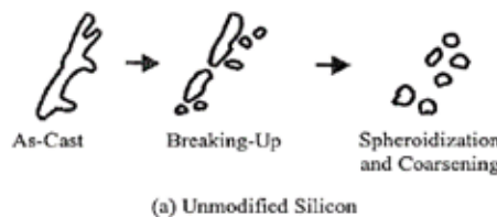
Figure 5: Silicon particles are broken down into smaller fragments and gradually spheroidized.
