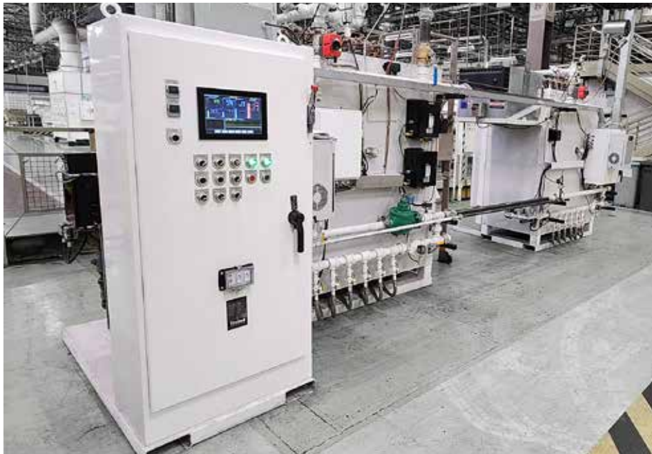
UPC-Marathon, a Nitrex company, replaced an outdated endo generator for an automotive manufacturer in Brazil. (Courtesy: Nitrex)
