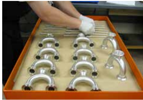
Solar Atmospheres Eastern PA specializes in the brazing of high-value components using filler metals based on nickel, silver, gold, and copper. (Courtesy: Solar Atmospheres)
