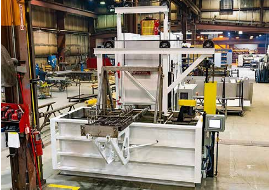
The maximum temperature for this Wisconsin Oven horizontal quench furnace is 1,200°F and the system has the capacity to heat 450 pounds of aluminum parts and the steel basket within 60 minutes. (Courtesy: Wisconsin Oven)
