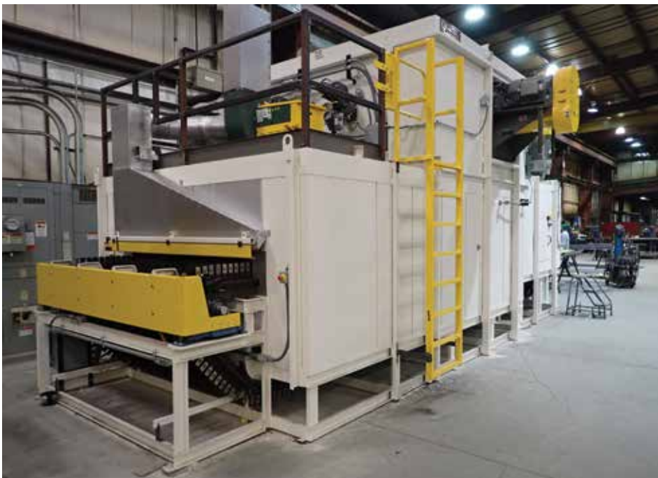
An electrically heated conveyor oven with forced air cooldown by Wisconsin Oven was shipped to an automotive manufacturer for use tempering automotive parts. (Courtesy: Wisconsin Oven Corporation)
