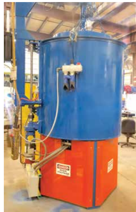
Lindberg/MPH has shipped an electrically heated steam atmosphere pit furnace for steam treating parts to a tooling manufacturer. (Courtesy: Lindberg/MPH)
