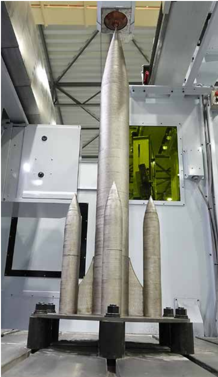
High-precision additive manufacturing means manufacturing a metal into an accurate shape with the proper mechanical properties. (Courtesy: Nidec)
