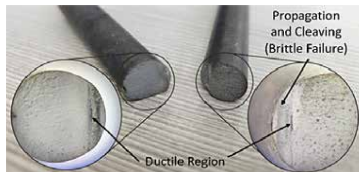
Figure 6: Tested sample, showing the fractured surface.
