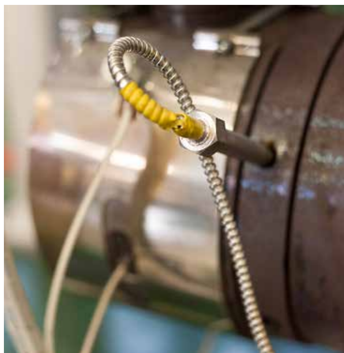
Figure 6: Temperature measurement accuracy is a function of all the elements in the system, not just the sensor. Transmitters and readouts also have an effect on total system accuracy.
