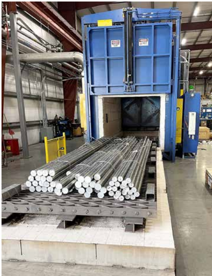
The new car bottom air furnace has a working zone that is 60-inches square by 168 inches long and handles a workload up to 30,000 pounds. (Courtesy: Solar Atmospheres of California)
