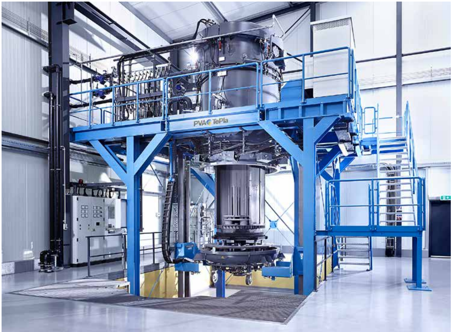
The furnaces that produce high-purity graphite also require components manufactured from graphite and related materials such as fiber-reinforced carbon. (Courtesy: PVA TePla America)
