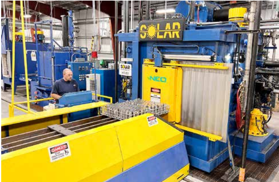
The NEO's vacuum chamber is designed to thermally heat parts with the use of work thermocouples, transferring into a vacuum protected vestibule within 20 seconds, and finally immersing a maximum 2,000-pound load into a hot agitated 3,000-gallon oil quench bath. (Courtesy: Solar Atmospheres)
