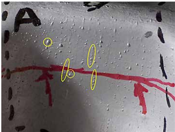
Figure 1: Appearance of blistering on 7075 forging.
