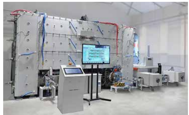
Figure 16: Single-piece flow vacuum furnace with LPC and with part dedicated HPGQ chamber [7].
