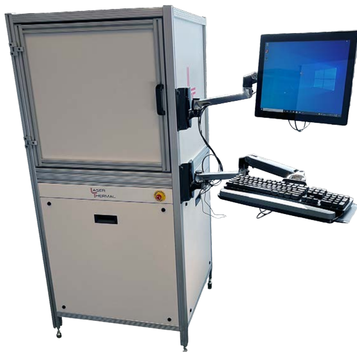
Laser Thermal has developed a method to measure the thermal properties of a material with a non-contact thermal conductivity measurement tool using optical technologies. (Courtesy: Laser Thermal)
