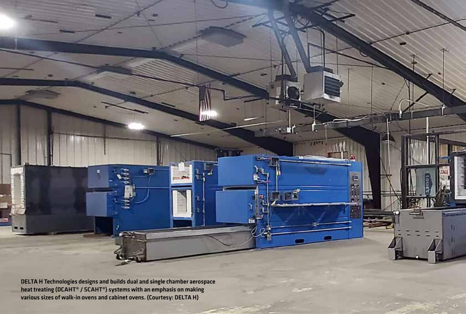
**DELTA H Technologies designs and builds dual and single chamber aerospace heat treating (DCAHT® / SCAHT®) systems with an emphasis on making various sizes of walk-in ovens and cabinet ovens. (Courtesy: DELTA H)**
