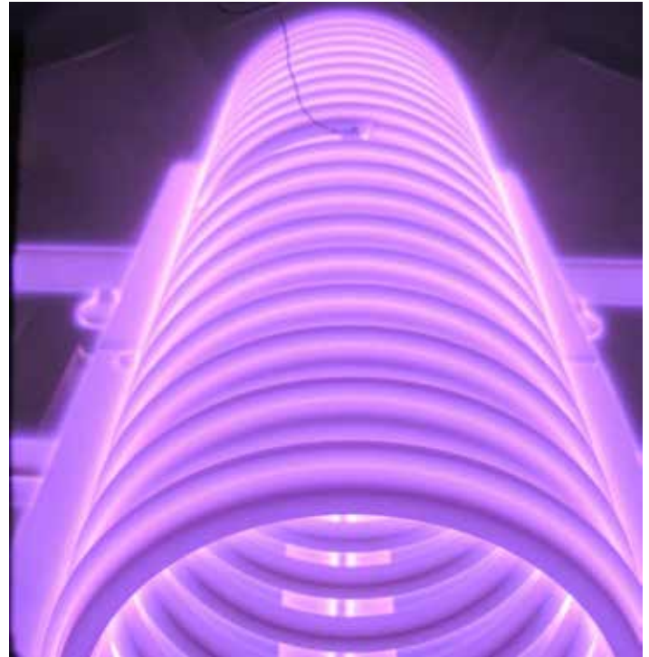
Figure 1: Plasma nitriding of stainless-steel rings. Image taken at Advanced Heat Treat Corp. Monroe, Michigan.
