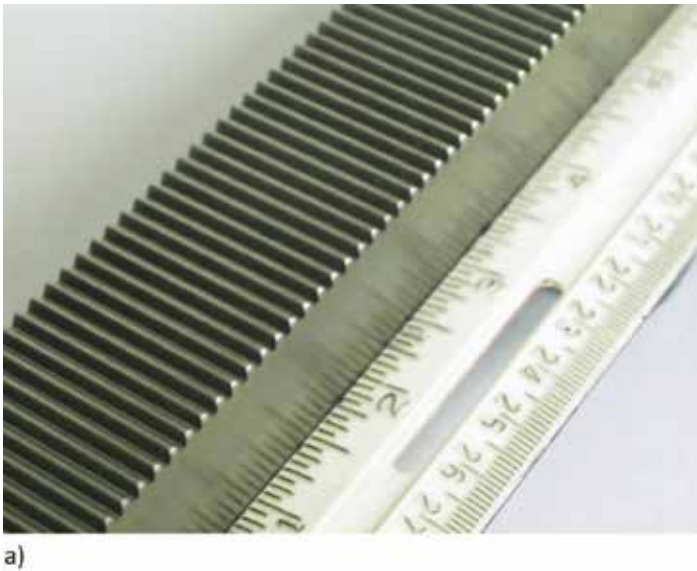
Figure 9: Plasma nitriding of rotors made of PM 316 SS. Image taken at Advanced Heat Treat Corp. Monroe, Michigan.
