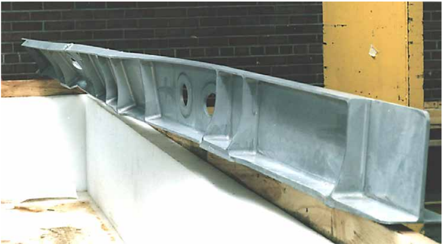
Figure 2: Distortion of an F/A-18 wing spar due to improper quenching and racking technique. Wing spar is 3,050 mm long.
