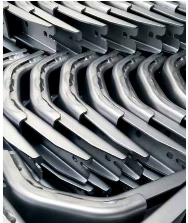
Aluminum parts are typically forged, cast, or formed prior to heat treatment. Each of these processes produce significant tensile or residual stresses. (Courtesy: Shutterstock)
