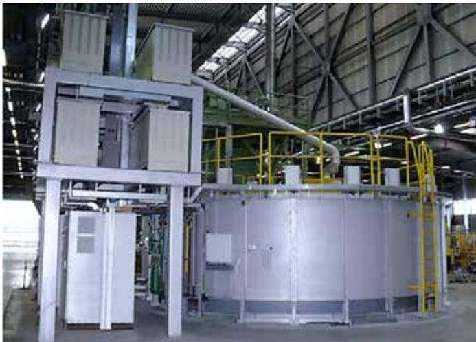
Figure 4: Rotary hearth atmospheric furnace.
