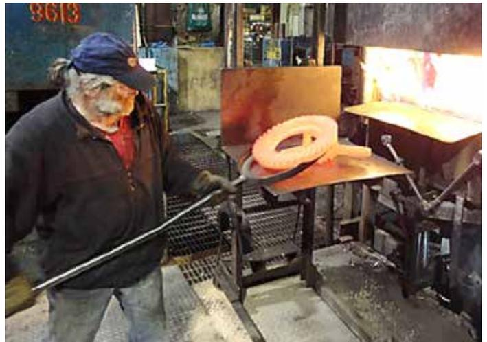
Figure 5: Manual transfer to press quenching.
