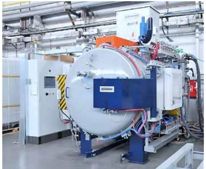
Figure 3: Vacuum furnace with batch HPGQ.
