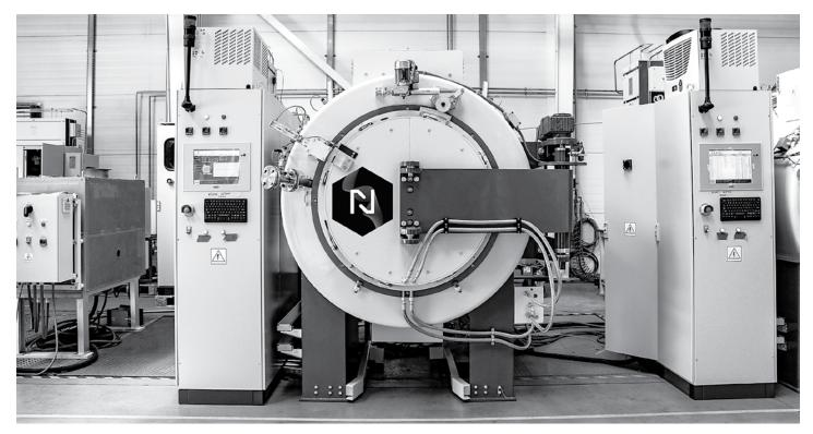
Nitrex's horizontal-type furnace, a model NXH-6612, can handle loads up to 800 kilograms (1,760 pounds). (Courtesy: Nitrex)
