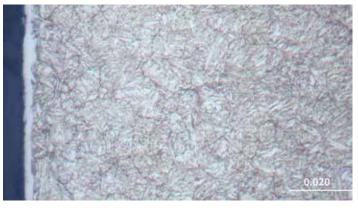
Figure 8: Photomicrograph of a typical near-surface zone in one of the samples. Nital etched. Note uneven thickness the compound zone, which demonstrate how difficult is to determine accurately its thickness.
