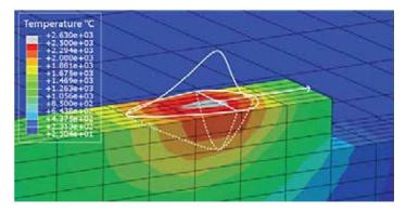
Figure 6: Goldak flux distribution overlaid on the temperature contour.
