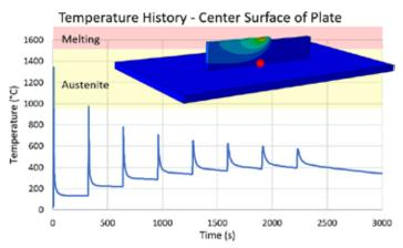
Figure 3: Temperature history for a point on the center surface of the build plate.
