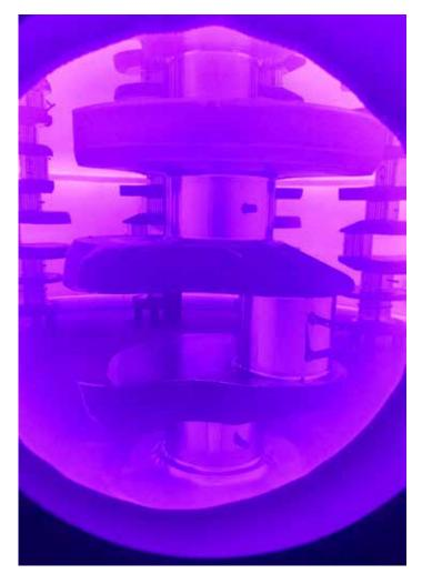
Figure 1: Preheating of the load of crankshafts with cathodic shields.
