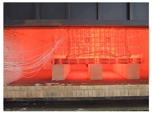
Temperature uniformity surveys (TUS): Depending on your furnace class or type of material you are processing, there are specific uniformity characteristics that must be met for your furnace to be certified to AMS 2750 – depending on its furnace class.
