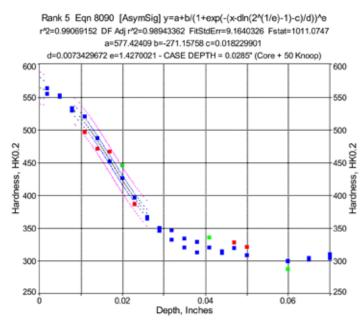
Figure 4: Hardness profile of the flat surface sample nitrided at 499°C /930°F in the "Base-Only."
