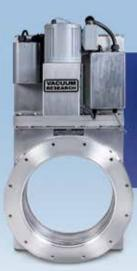
All VRC Motor Actuators Provide Open/Close, Throttle, and Soft Start Using Your Existing PLC with 0 to 10 VDC or 4-20 mA Output.
