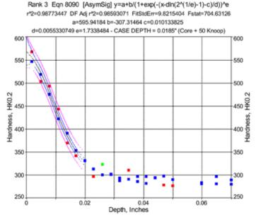
Figure 10: Hardness profile of the flat surface sample nitrided at  $460^{\circ}C$  ( $860^{\circ}F$ ) in the "Base & Shields" mode, as tested by Person 1.
