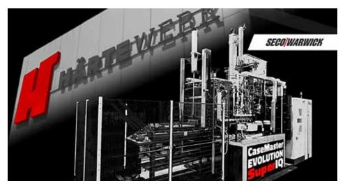
The Seco/Warwick system ordered by Härtewerk Chemnitz GmbH – the Super IQ – is a two-chamber vacuum furnace with oil or gas quenching and low-pressure carburizing. (Courtesy: Seco/Warwick)
