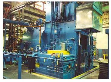
Figure 1: Typical integral quench furnace (Courtesy: Surface Combustion, Maumee, Ohio).
