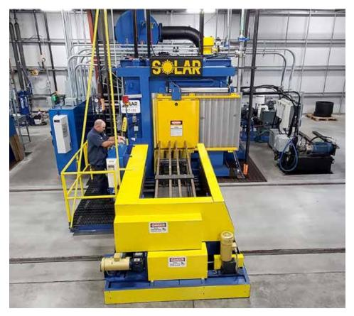
Solar Atmospheres of Western PA's two-chamber VOQ furnace is completely sealed, meaning a significantly cleaner and safer oil quenching process. (Courtesy: Solar Atmospheres of Western PA)
