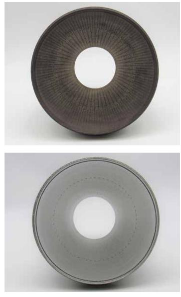
As-printed/heat treated image (top) and after REM Surface Engineering's Extreme ISF® Process image (bottom) of a LBP-DED rocket nozzle. (Courtesy: NASA MSFC)
