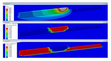
Figure 4: Temperature (top) and phase fractions of austenite (middle) and pearlite (bottom) during the second deposition pass.
