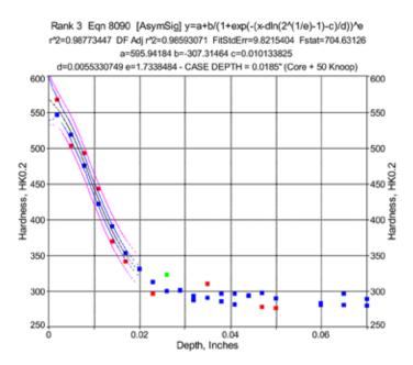
Figure 9: Hardness profile of the round surface sample nitrided at 460°C (860°F) in the "Base & Shields" mode, as tested by Person 1.
