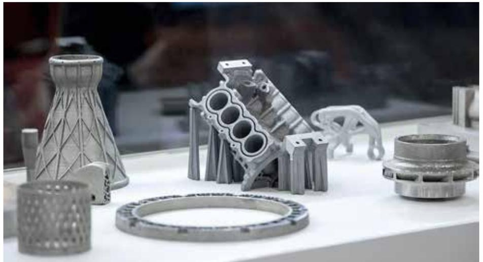
**If an AM part is integral to a safety critical aerospace or medical application, it is essential to achieve dimensional and material tolerance targets consistent with design intent. (Courtesy: ZYGO)**
