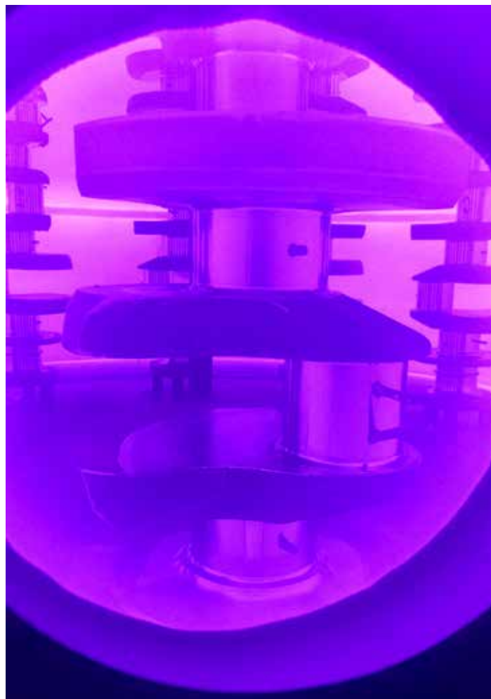
Figure 1: Preheating of the load of crankshafts with cathodic shields.
