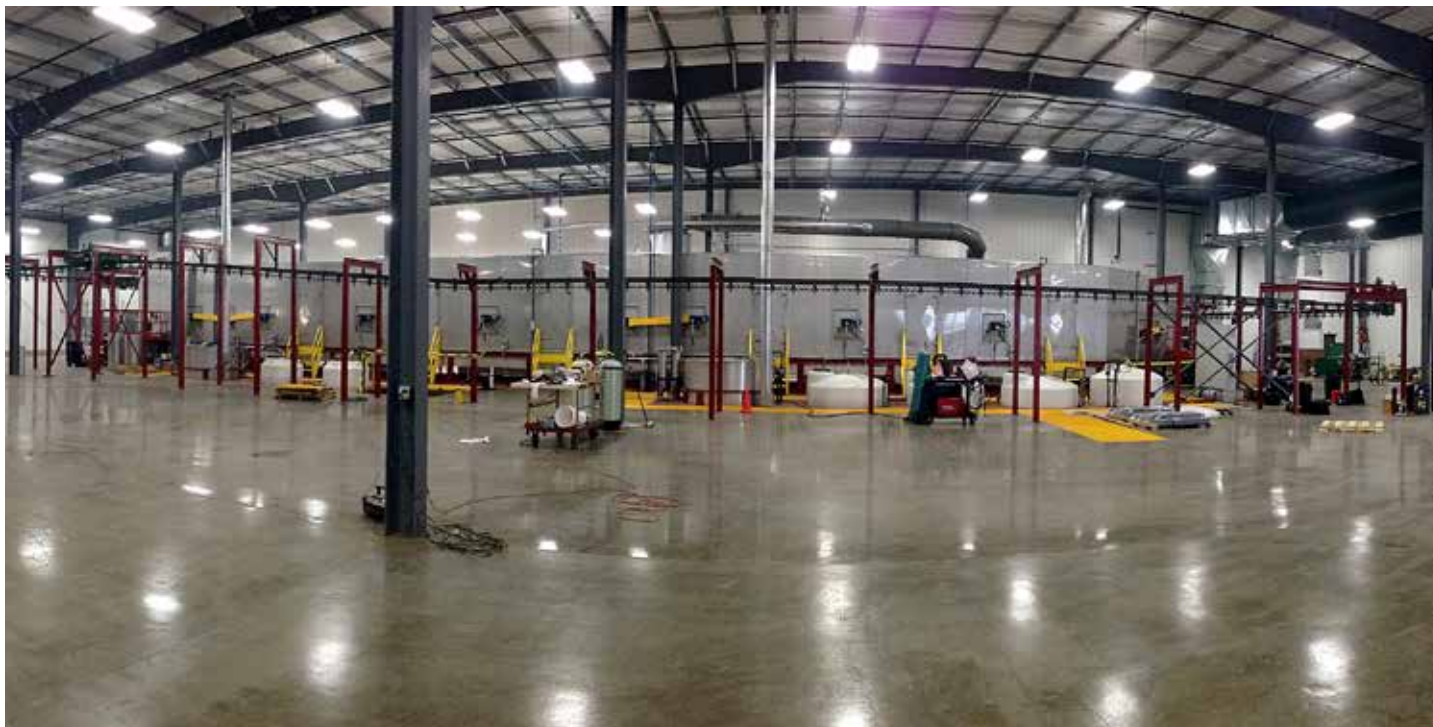
A finishing system washer using torrent washer technology. (Courtesy: Horizon Performance Technologies)
