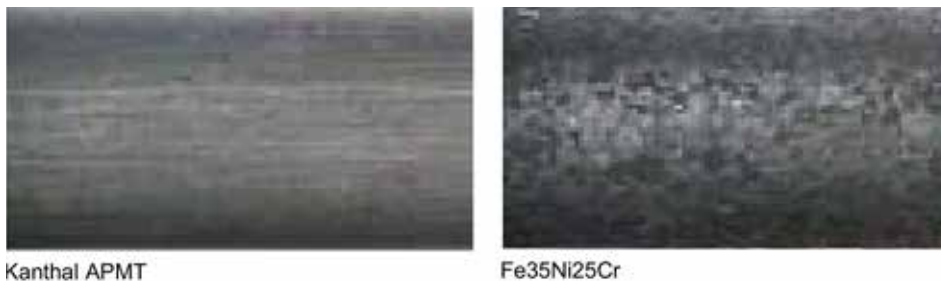
Figure 1: Oxidation property of Kanthal APMT VS. Fe35Ni25Cr.
