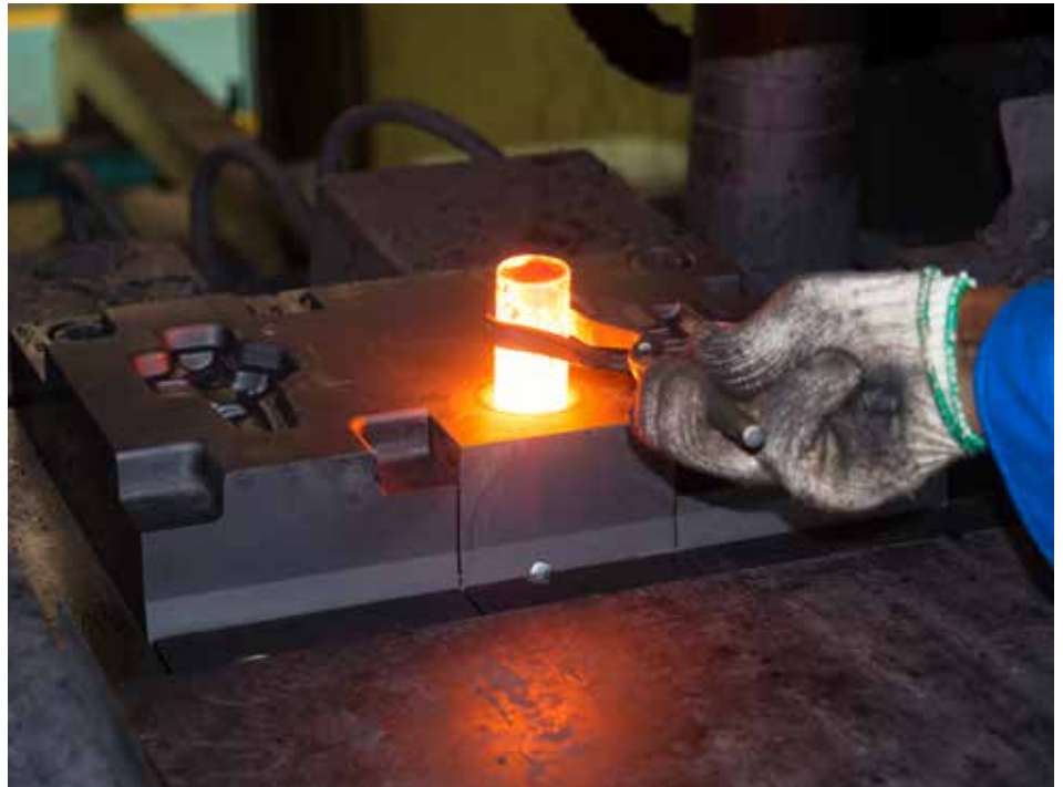
Although nitrided hot working tools are very brittle and tend to crack due to the thermal and mechanical stresses during forging, the average tool life of nitrided tools is about 40 percent higher than that of tools that have only been quenched and tempered. (Courtesy: Shutterstock)
