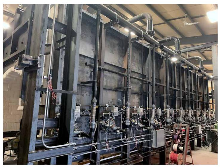
A 20-burner 20M BTU 1,750°F construction car bottom furnace in production. (Courtesy: Noble Industrial Furnace)
