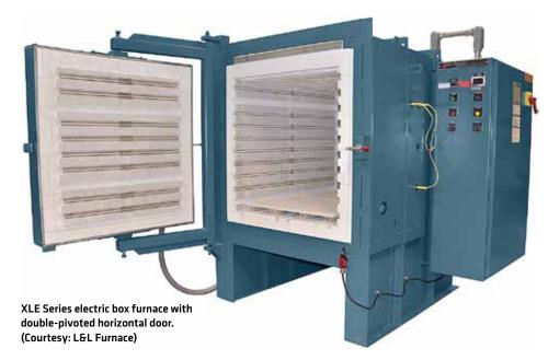
The control system is driven by a Honeywell program control with an over-temperature control to prevent the furnace from overfiring. A digital round single-input chart recorder keeps accurate recordings of the furnace process temperature. The Kanthal Iron Aluminum Chrome coiled elements located on the sides, back, and door are controlled in two zones for balancing of temperature gradients from top to bottom.
