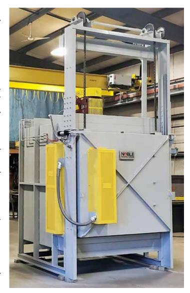
A 90 kW electric box furnace with rod-overbend elements and a circulation fan allowing for processing temperature range of 700-1,650°F. (Courtesy: Noble Industrial Furnace)
