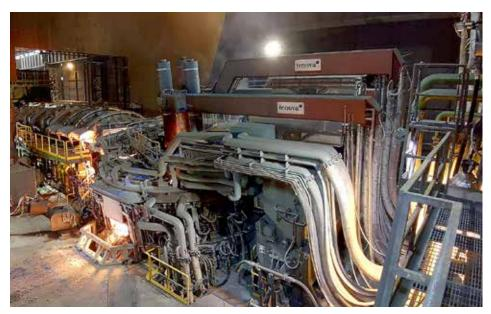
ABB and Tenova receive final acceptance for innovative charging, melting and electromagnetic stirring solution on a large electric arc furnace. (Courtesy: Tenova)
