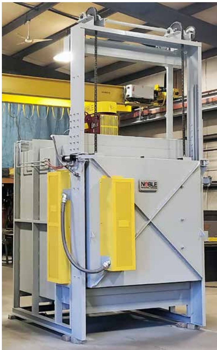
A 90 kW electric box furnace with rod-overbend elements and a circulation fan allowing for processing temperature range of 700-1,650°F. (Courtesy: Noble Industrial Furnace)
