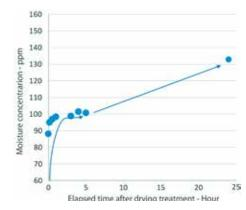
Figure 4: Change in moisture in AI alloy powder after drying.
