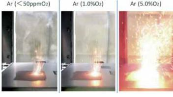
Figure 7: Spatter under various % oxygen contamination.
