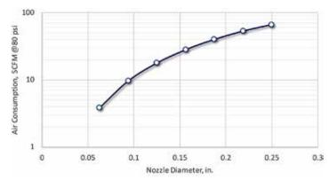
Figure 1: Air consumption of simple nozzles, based on hole diameter in pipe [4]
