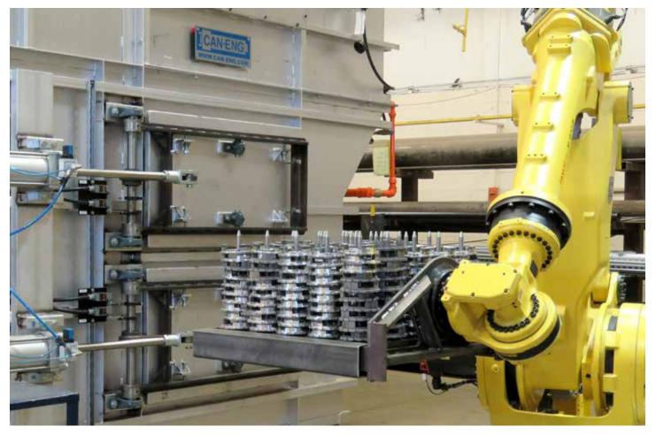
For the past 15 years, Can-Eng has been integrating robotic handling in its aluminum heat-treat systems. (Courtesy: Can-Eng)
