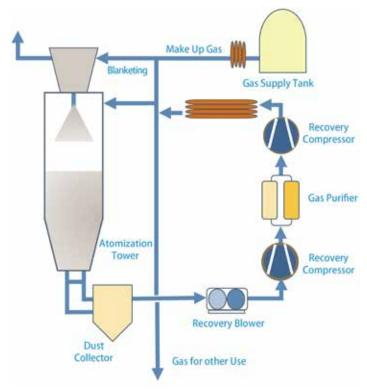
Figure 2: Gas recycle system in metal powder production.
