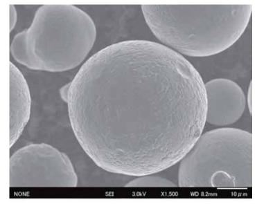
Figure 1: Metal powder under 1,500X magnification.
