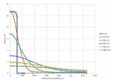
Figure 4: Pattern spread and velocity profile of a 25-mm submerged jet nozzle, using water at 20C, as a function of distance from the exit of the nozzle.
