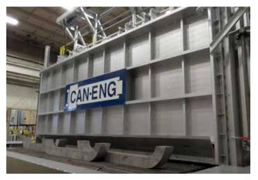
An aluminum-conveyor furnace. (Courtesy: Can-Eng)
