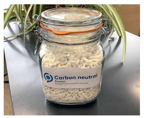
Figure 5: Fully calcined Ultralite loose fill granules (prill).
