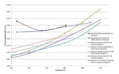
Figure 4: Thermal conductivity chart showing Ultralite against alternative products (kiln firing ceramic sanitaryware).
