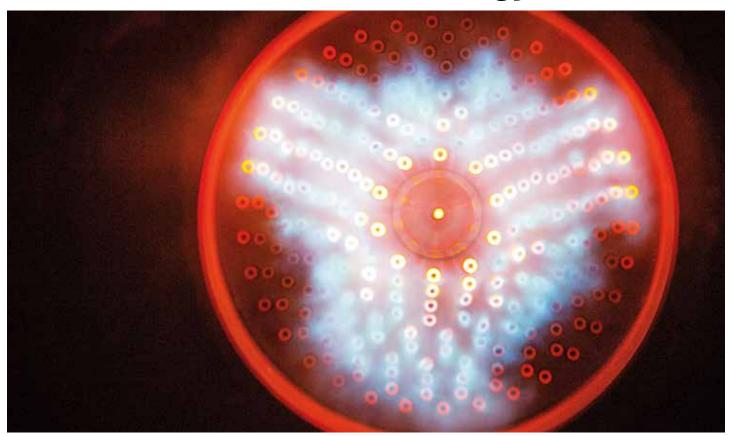
WS is also known for inventing the game-changing flameless oxidation (FLOX®) technology, which enables high-combustion efficiency with low NOx emissions.
