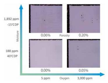
Figure 8: Effect of oxygen and moisture on porosity.
