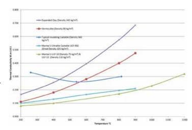
Figure 3: Thermal conductivity chart showing Ultralite against alternative products (kiln firing heavy clay).
