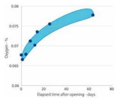
Figure 3: Change in oxygen in AI alloy powder after opening.
