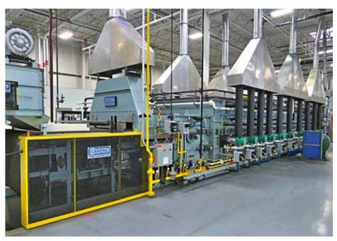
A mesh-belt furnace. (Courtesy: Can-Eng)
