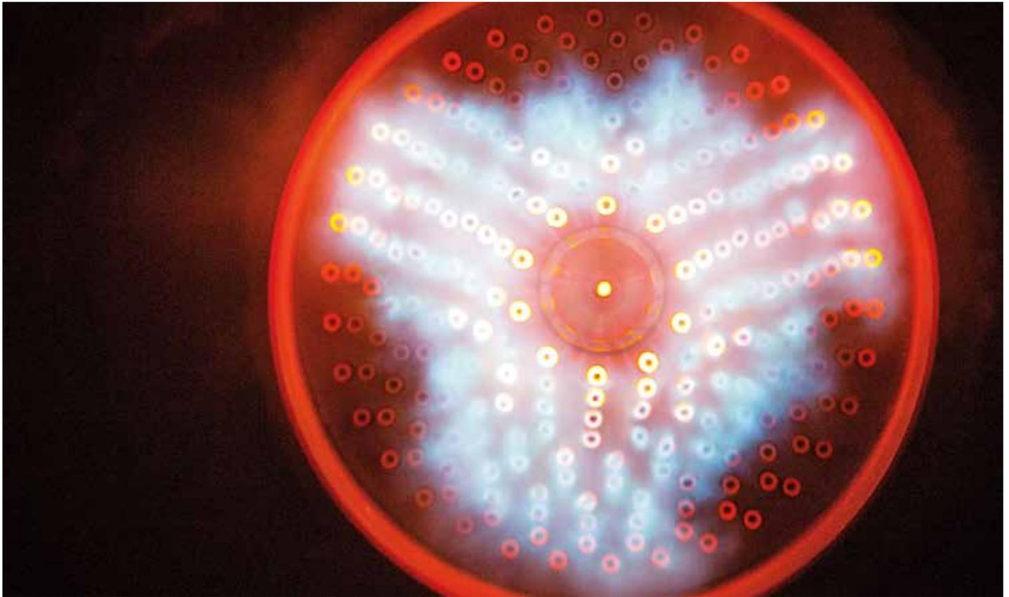
WS is also known for inventing the game-changing flameless oxidation (FLOX<sup>®</sup>) technology, which enables high-combustion efficiency with low NOx emissions.
