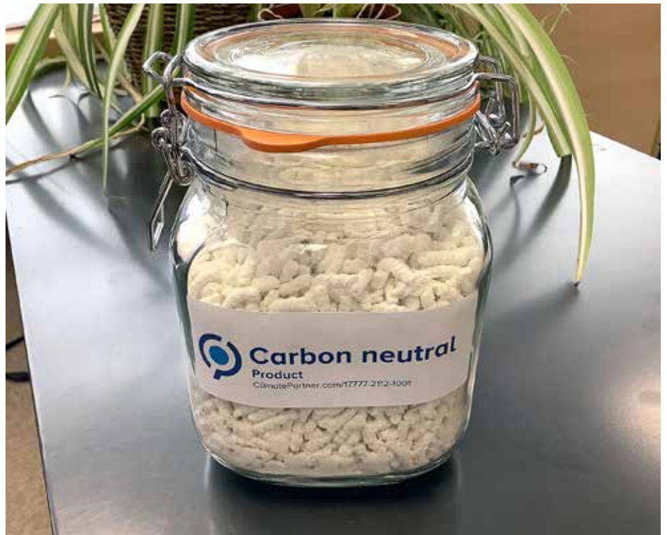
Figure 5: Fully calcined Ultralite loose fill granules (prill).
