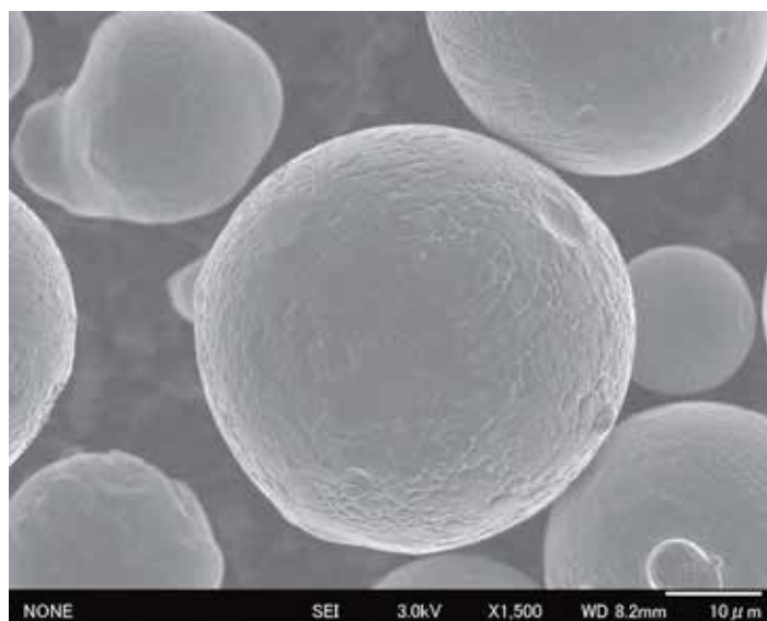
Figure 1: Metal powder under 1,500X magnification.
