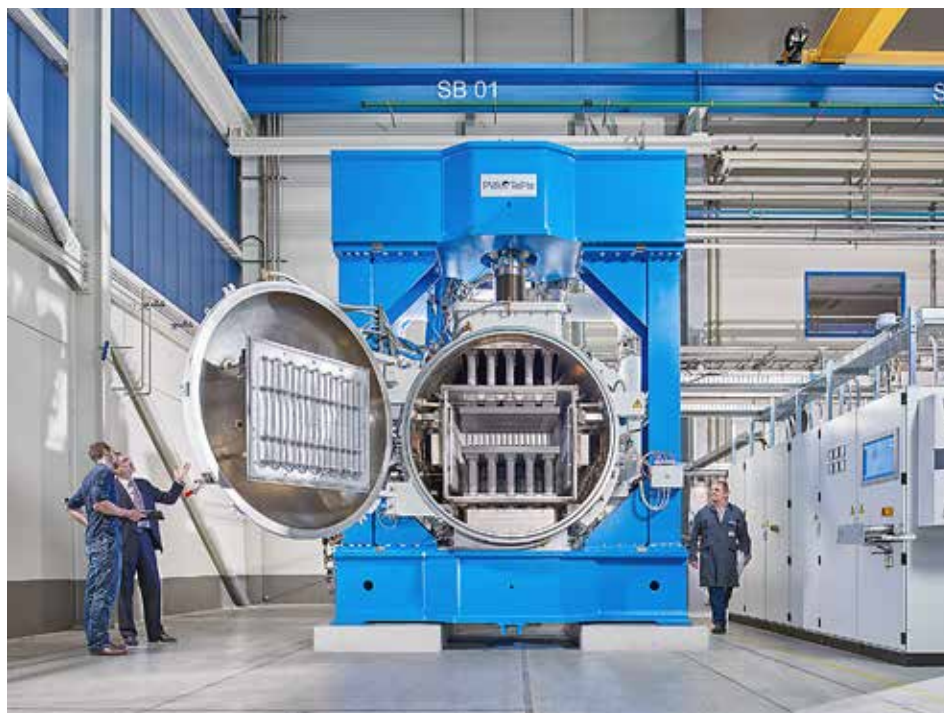
The concept is to bond layers of sheet metal that contain machined channel/microchannel structures. (Courtesy: PVA TePla America)
