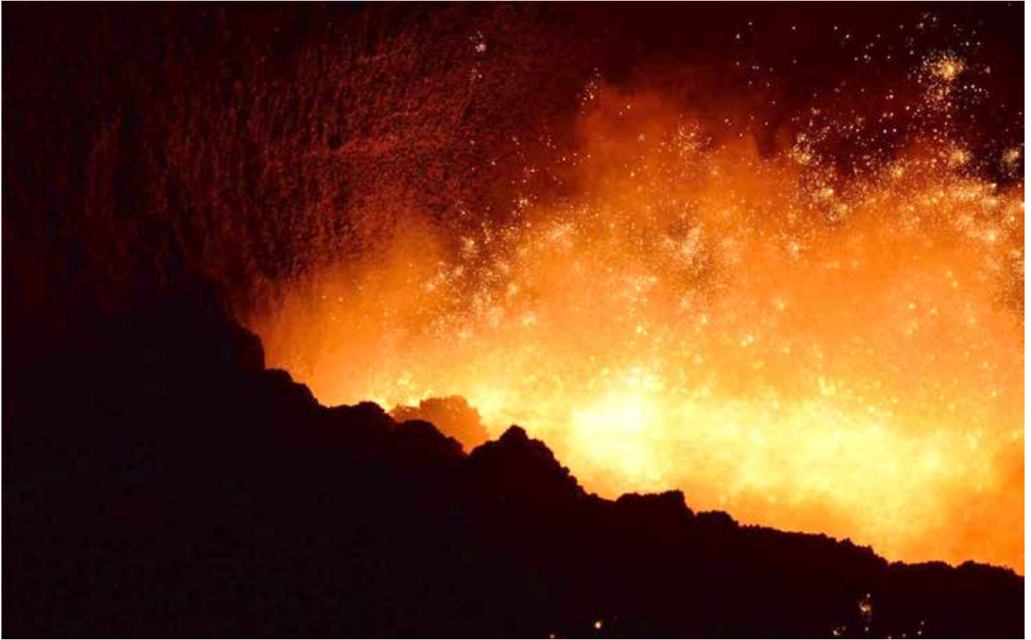
Figure 5: Offgas, sparks, and airborne liquid: blast furnace taphole at casting.
