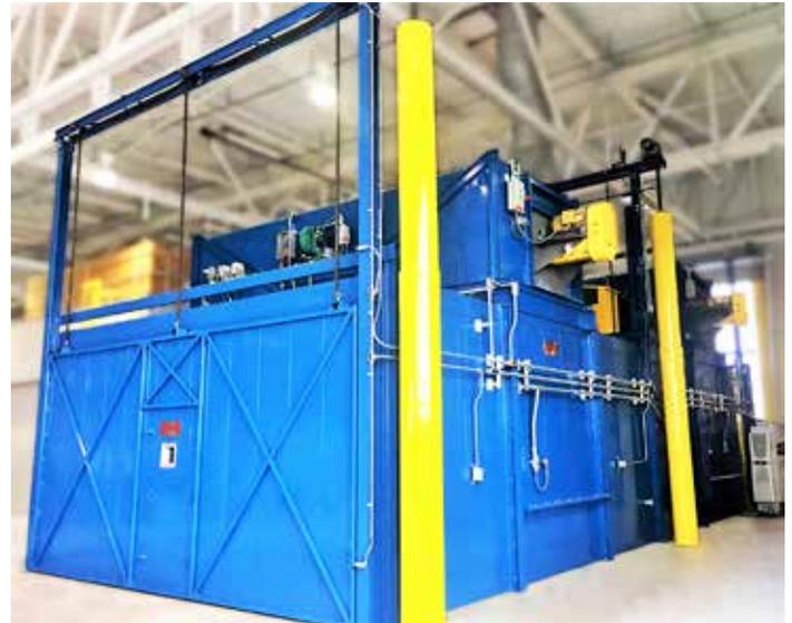
Installed batch aerospace oven equipped with pneumatic guillotine doors and integrated air pollution control units. (Courtesy: Epcon Industrial Systems)
