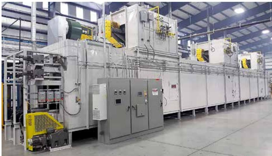
**Automated coil coating line featuring a control panel for the precision of air flow management and temperature control modules. (Courtesy: Epcon Industrial Systems)**
