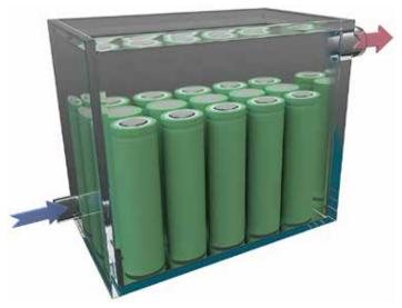
Figure 7: This schematic shows the benefits of direct cooling where the heat-transfer fluid is in direct contact with the battery and electronics. (Courtesy: The Lubrizol Corp.)
