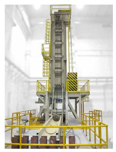
A VertiQuench® Solution HT and aging drop bottom type furnaces. (Courtesy: SECO/WARWICK)
