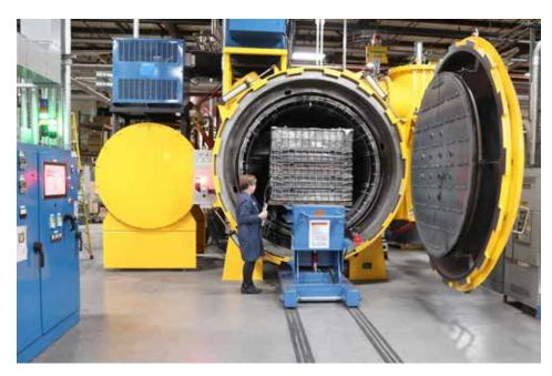
The vacuum furnace installation incorporates Solar Manufacturing's latest and most advanced vacuum furnace technology, aimed at safety and efficiency. (Courtesy: Solar Atmospheres)
