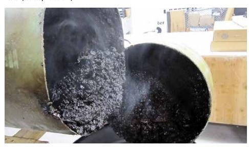
Figure 2: Heat-transfer fluids can oxidize during use, which will lead to premature failure as shown by this image of a sludged expansion tank. (Courtesy: Duratherm)
