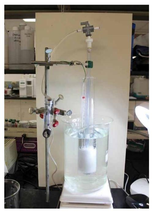
Figure 3: The experimental setup for evaluating the foaming of a water-glycol heat-transfer fluid using ASTM D1881 is shown. (Courtesy: Dynalene)
