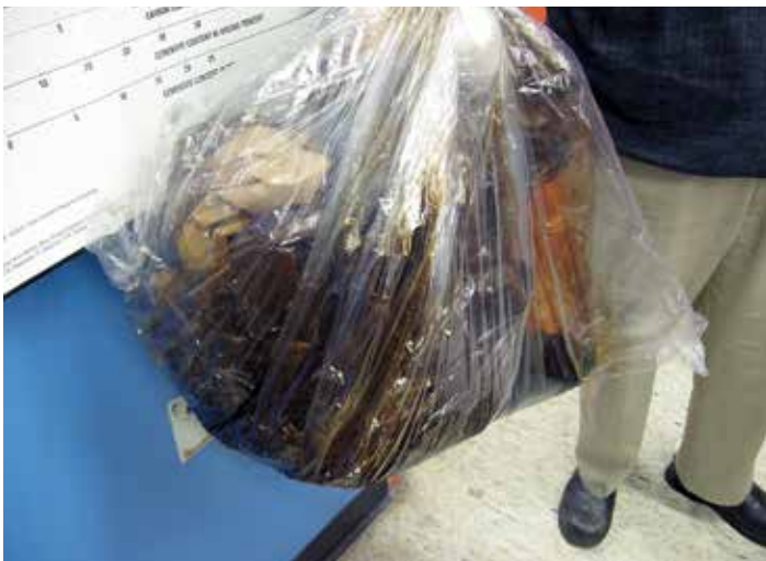
Figure 4: A poorly packed sample as it arrived for testing. The carrier provided the bag because the package contents spilled during shipment. No lid locks were provided.
