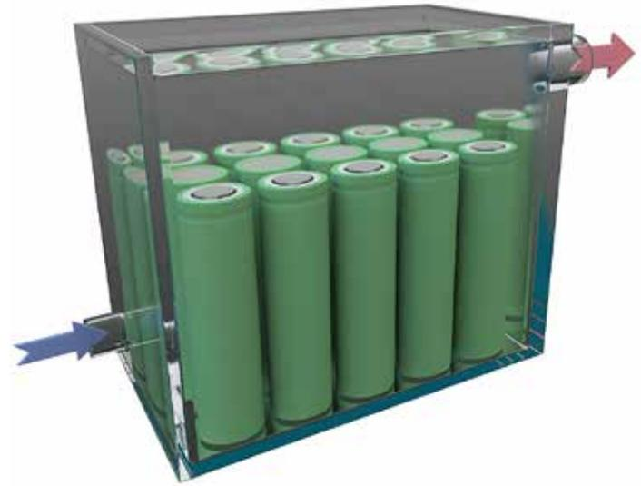
**Figure 7:** This schematic shows the benefits of direct cooling where the heat-transfer fluid is in direct contact with the battery and electronics. (Courtesy: The Lubrizol Corp.)
