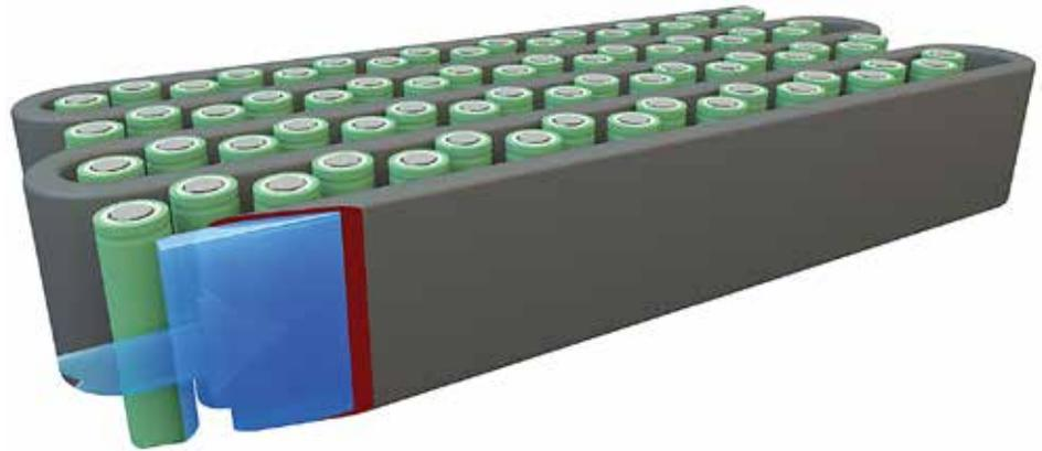
**Figure 8:** A schematic shows the indirect cooling method known as side cooling. (Courtesy: The Lubrizol Corp.)
