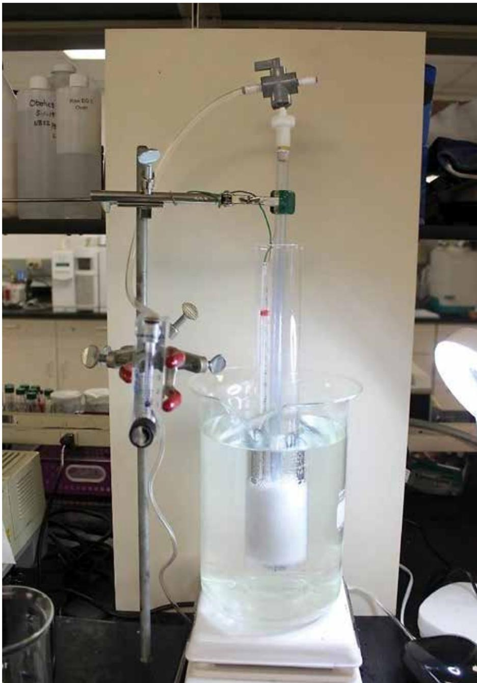
**Figure 3: The experimental setup for evaluating the foaming of a water-glycol heat-transfer fluid using ASTM D1881 is shown. (Courtesy: Dynalene)**
