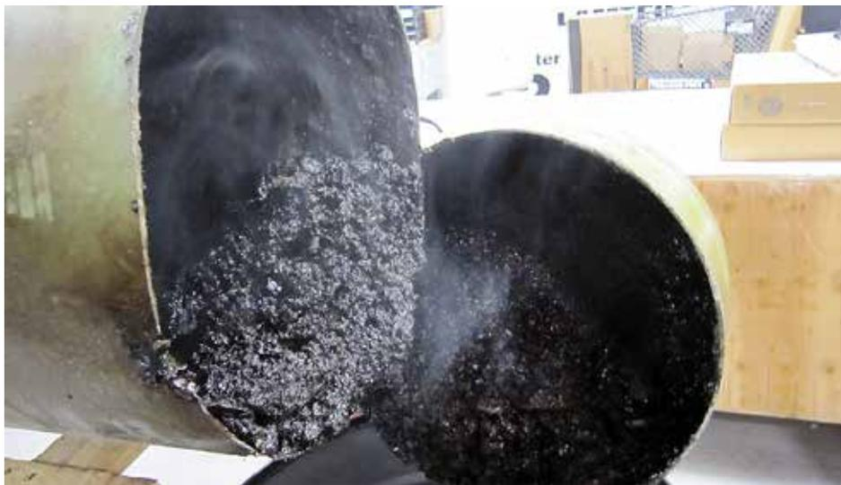
Figure 2: Heat-transfer fluids can oxidize during use, which will lead to premature failure as shown by this image of a sludged expansion tank. (Courtesy: Duratherm)
