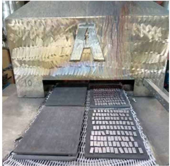
Figure 1: Photo of TRS bars entering conventional furnace. Single-layer loading on the right, double-stack loading on the left.
