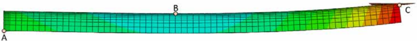
Figure 2: Beam showing distortion modes of a bevel gear tooth.
