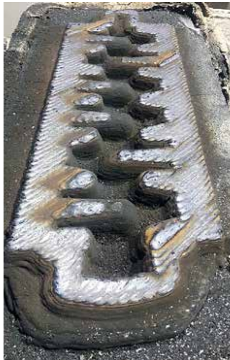
Crankshaft die welded with a robot. (Courtesy: COR-MET)
