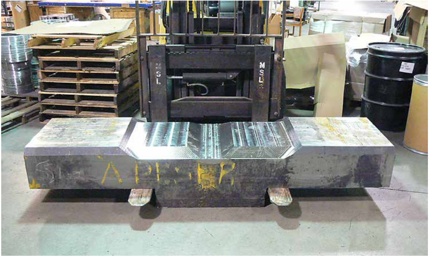
Flat die machined ready for welding. (Courtesy: COR-MET)
