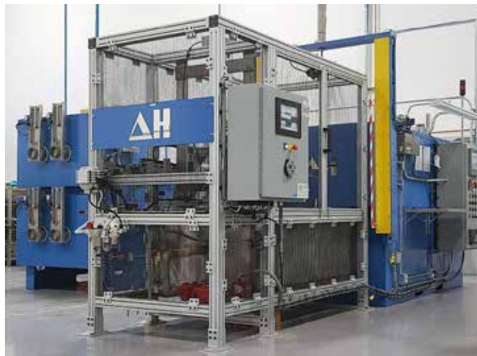
DELTA H® SCAHT® and DCAHT® fully automated AM and aerospace aluminum heat treating at Burloak Technologies. (Courtesy: Delta H Technologies)
