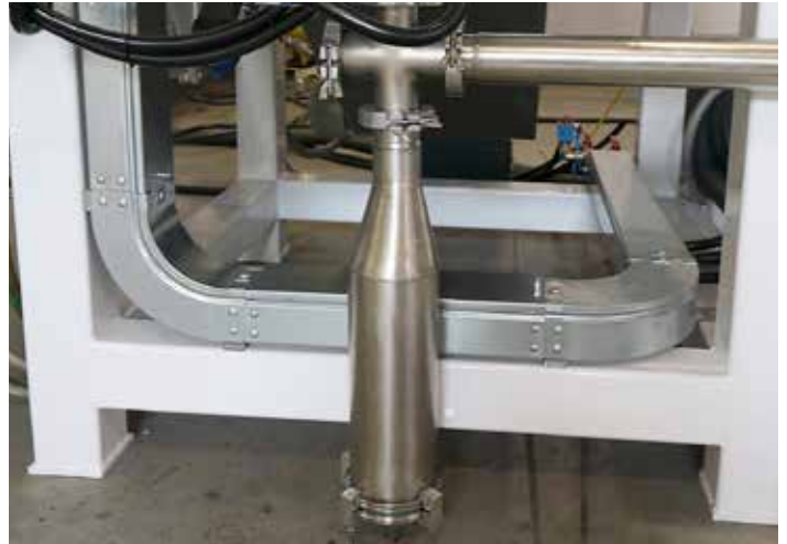
The storage tank. (Courtesy: TAV VACUUM FURNACES)
