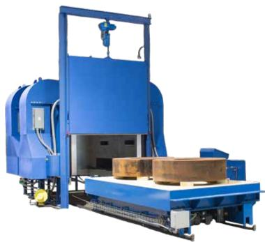
A car-bottom furnace. (Courtesy: Applied Test Systems)
