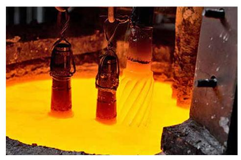
Parts that are heated in salt baths are heated by conduction. The thermal mass of the molten salt provides a large thermal source for heating of parts.
