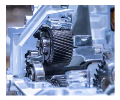
EV powertrain components must be strengthened to withstand the additional loads and stresses, enhancing metallurgical properties, yet minimizing distortion and noise characteristics.
