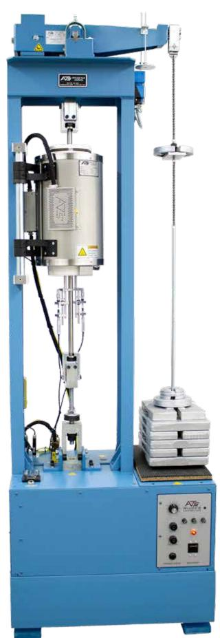
ATS performs creep testing. (Courtesy: Applied Test Systems)
