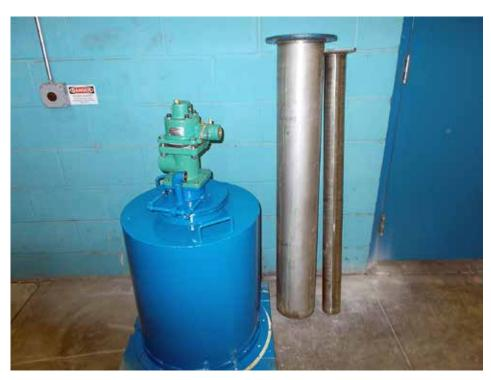
Figure 1: Endocarb unit with burner, retort, and burner tube.
