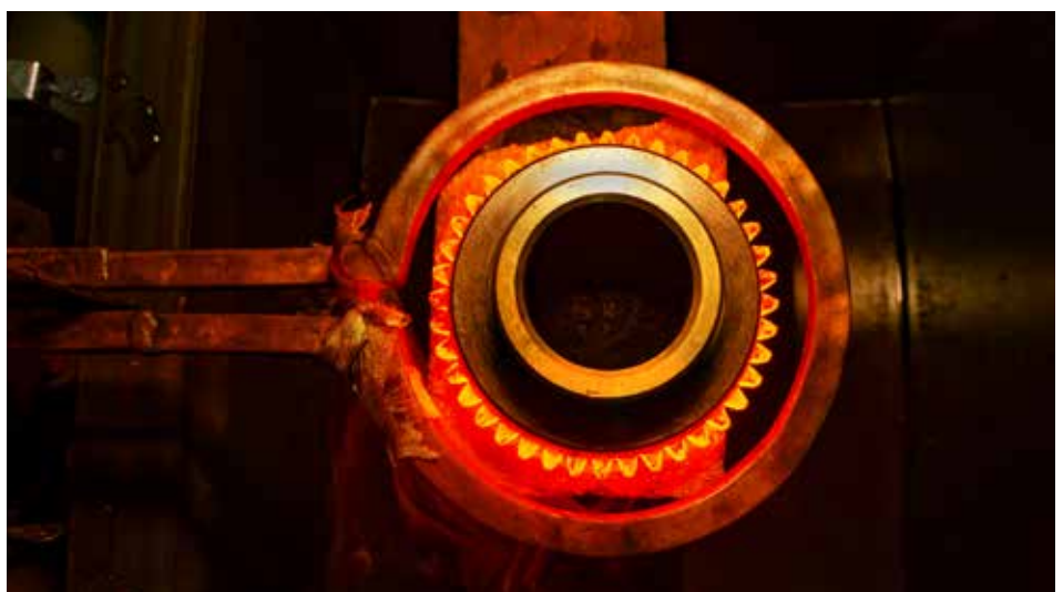
Figure 2: Cross-sectional temperature profile of a 50 mm (2-inch) bar created using induction heating and simultaneously cooling during heating.
