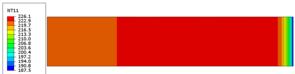
Figure 2: Cross-sectional temperature profile of a 50 mm (2-inch) bar created using induction heating and simultaneously cooling during heating.
