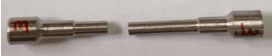
Figure 10: Sample THA-1 with THA-3 fractured in the zone distant from the joint line material THA-3.
