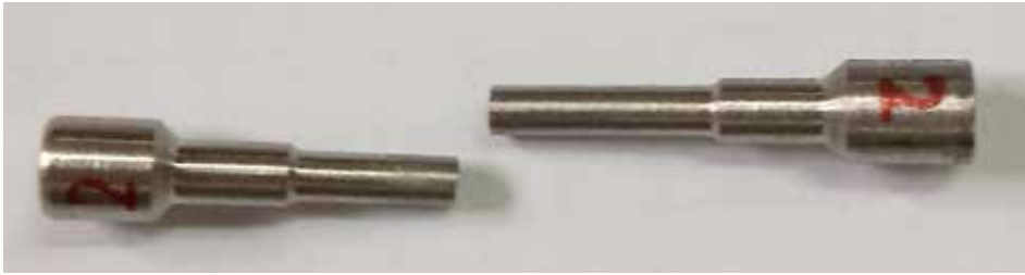
Figure 9: Sample THA-2 with THA-3 fractured in the joint line or in its immediate vicinity.
