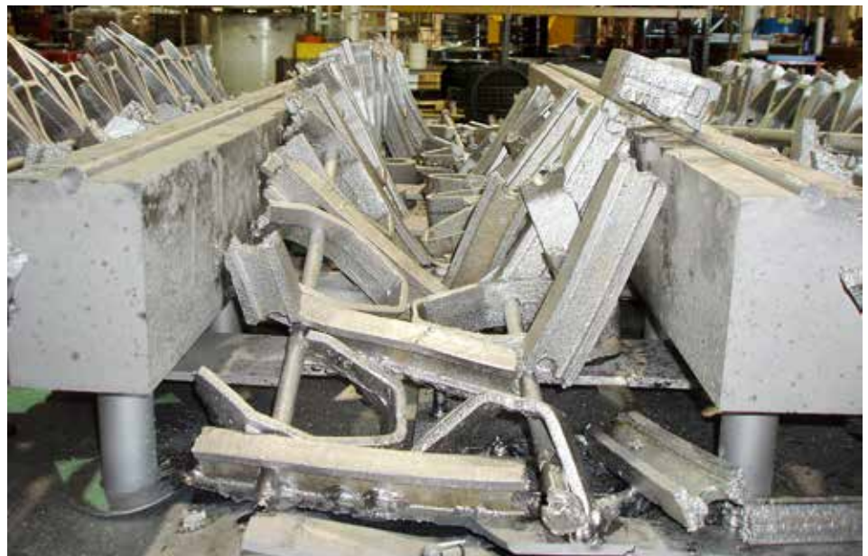
Figure 1: Eutectic meltdown between the high nickel alloy cast fabrication grid and the molybdenum load rods. This was an expensive mistake, in excess of $150,000. (Courtesy: Solar Atmospheres, Inc.)
